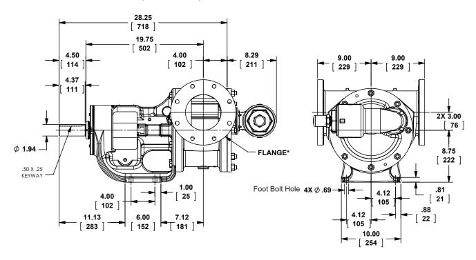
\*NOTE: Flanges are 6", suitable for use with Class 150 ANSI steel or stainless steel companion flanges or flanged fittings.
