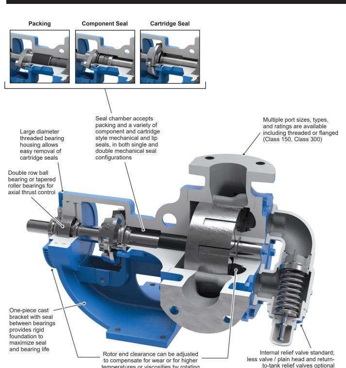
temperatures or viscosities by rotating the threaded bearing housing
