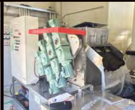
Mixed Sludge at Confectionary Plant (JD-500)
